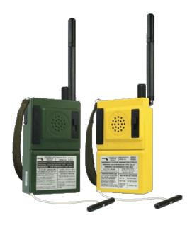
The Series 500-27 Personal Locator Beacons are simple, compact lightweight units which can be used either manually or automatically via ejection seat harness. A fully embedded 12 channel GPS with data burst transmission on 406.025 MHz. Fully compatible with the majority of search and rescue equipment including the COSPAS/SARSAT satellite based survivor location equipment.
