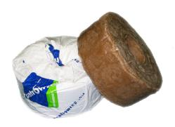
PetroWrap Anti-Corrosion Tape consists of a non-woven, stitch bonded, synthetic fabric which has been fully impregnated with neutral petrolatum based compounds and inert fillers. PetroWrap Anti-Corrosion Tape will not crack, peel, or harden and therefore remains impermeable to moisture and requires no maintenance. PetroWrap ensures easy site application with-out heating, even in the coldest temperatures, and can be applied on damp and indifferently prepared surfaces.
