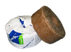
PetroWrap Anti-Corrosion Tape consists of a non-woven, stitch bonded, synthetic fabric which has been fully impregnated with neutral petrolatum based compounds and inert fillers.
