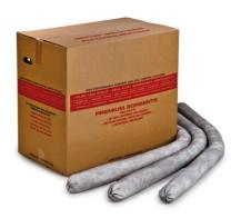
The socks feature a tough *spun-bond* outer sleeve that has a durable *heat sealed seam* running its entire length. This tube is then filled with a *super absorbent foam core* that is *made from 100% post industrial material*. The super absorbent core is secured into the sleeve at each end with a durable metal clip.
