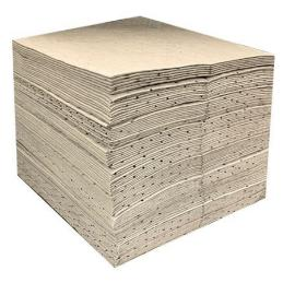
The pads are made from a single layer of meltblown which is sonically bonded together. The sonic bonding points make the pad less prone to stray fibers becoming detached. This gives the pad a very even structure which also contributes to the pad's good absorbency rate. These attributes help make the pad an industry standard construction because it offers all-round average performance but excellent versatility.
