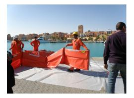
Harbor oil containment boom is commonly used for dockside operations. Also called layflat boom, it is designed with rectangular flotation and a flexible fabric skirt which limits storage requirements. ABASCO harbor oil spill booms are available in several sizes and strengths (see below) to contain spills in conditions from quiescent waters to harbor applications.
