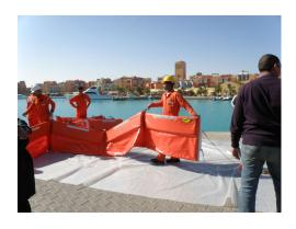
Harbor oil containment boom is commonly used for dockside operations. Also called layflat boom, it is designed with rectangular flotation and a flexible fabric skirt which limits storage requirements. ABASCO harbor oil spill booms are available in several sizes and strengths (see below) to contain spills in conditions from quiescent waters to harbor applications.
