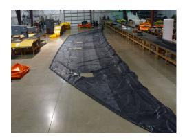
ABASCO heavy duty diversion baffles are ideal for controlling flow and circulation in wastewater treating ponds, to eliminate dead zones, increase detention time, and improve treatment efficiency. Heavy duty tension members at the top and bottom of the curtain and UV/chemical/acid/base resistant 30 oz. Elvaloy coated fabric with additional skirt fabric options. Custom design upon request including high wind conditions.
