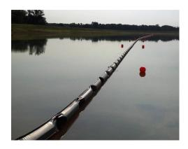
ABASCO light duty floating diversion baffles are ideal for controlling flow and circulation in wastewater treating ponds, to eliminate dead zones, increase detention time, and improve treatment efficiency. Tension member is a ballast chain at bottom of the curtain skirt. Standard fabric is a 35oz PVC fabric with options a permeable skirt or upgraded UV resistant 30 oz. Elvaloy coated fabric. Custom design options upon request.
