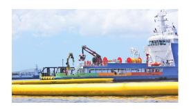
The NOFI Spill Raider is the most advanced offshore automatic inflatable oil containment boom available, developed with focus on operational safety, fast deployment and greater versatility. The NOFI Spill Raider is designed with focus on operational efficiency i.e. deployment speed, inflation method, less manpower needed and wave following characteristics.
