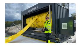
The ECOSPEED booms are air-filled containment booms which expand instantly as they come off the reel during deployment, without the need of blowers, compressors, or other forms of external air-supply. Instead, air is sucked in through the flushmounted breathers situated on the top of the boom, thereby filling the floats with atmospheric air. The self-inflating system and absence of check valves make the ECOSPEED an exceptionally fast launching boom, with minimum personnel requirements.
