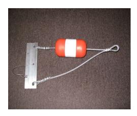
Available from 3" to 25". Attached to turbidity curtains to distribute the load exerted by towing or anchoring the curtain. Includes one aluminum connector, ASTM pin, plastic float, and 5/16" galvanized aircraft cable.
