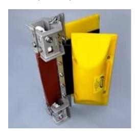
ABASCO's Tide Risers allow the boom to rise and fall during tidal fluctuations to maintain optimum draft. Rollers glide along a beam attached to a bulkhead or other permanent structure. The primary application is for SIGMA permanent boom installations, but tide risers can also used with conventional soft boom.
