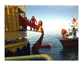
NEO Boom is a strong, durable boom that combines the compactability of an air-inflated boom with all the benefits and strength of a boom having conventional foam flotation. The product has been proven over years to be a cost-effective solution where storage space is limited but the application requires a durable containment boom. Ease of deployment, excellent wave conformity, and high buoyancy-to-weight ratios are key NEO Boom benefits.
