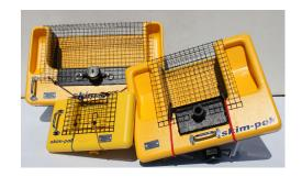
ABASCO offers a wide variety of weir style skimmers suited for numerous applications in both oil spill and industrial applications. The weir skimmers require either a suction pump or vacuum system to collect the free floating hydrocarbons or other materials. Weir skimmers are designed for easy portability, rapid response and low cost removing floating oil that can flow over the weir.
