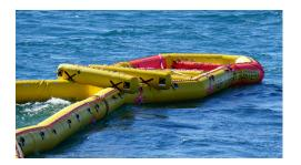
The NOFI Current Buster® 6 is currently in use by many oil spill control organizations all over the world. Offers excellent area coverage and flexibility in towing speeds up to 5 knots. The system is available in a number of different storage options, from hydraulic reels to containerized all-in-one alternatives. The NOFI Current Buster® 6 is well suited for single-vessel operations when used together with the BoomVane system.
