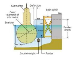
TekMarine TJHF Hydropneumatic Fenders are designed for vessels, such as submarines, that make contact with fenders below the waterline.
