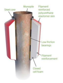
TJDF Donut Fenders guide vessels at lock entrances, berth approaches and turning points. The donut floats around a tubular pile and follows changes in the water level.
