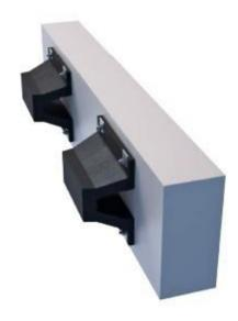
TJDA-A Arch Fenders are single piece rubber units. The simplest version has a plain rubber face and can be installed almost anywhere. An optional embedded steel plate allows mounting behind pilings, or for UHMW-PE facings (p28) or steel plates to be attached.
