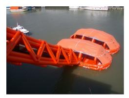
Liferaft Systems Australia (LSA) range of Marine Evacuation Systems (MES), provide rapid and safe evacuation which delivers passengers and crew, dry-shod, directly into large capacity liferafts.
