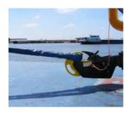
The GSH towing hook offers flexibility in operation, with both manual and remote release options available. Its intuitive design allows for effortless manual operation, requiring minimal exertion even at full capacity. Featuring a robust two-step release mechanism, accidental openings are effectively prevented, guaranteeing peace of mind during towing maneuvers.
